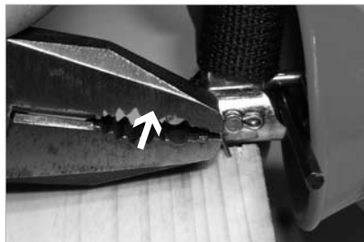
Fig. 15f Place the end of the pin on a suitable edge, e.g. on a wooden board as shown above, and bend the pin over the edge as far as it goes.
