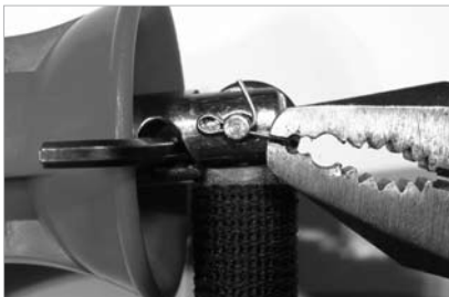
Fig. 15e Now take hold of the straight end of the cotter pin with the pliers (as shown in the illustration).
