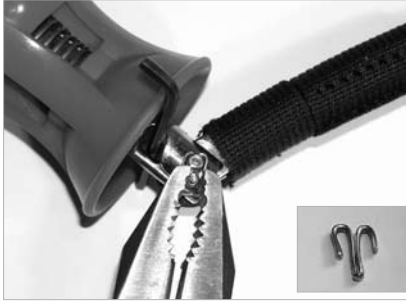
Fig. 14A Push the release grip up and secure it with the Allen key. Flatten the head of the cotter pin with a pair of flat nose pliers. (see small image).
