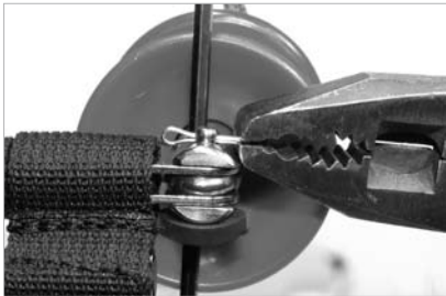
Fig. 15c Take hold of the long end of the cotter pin and pull it upwards with the help of a pair of flat nose pliers.
