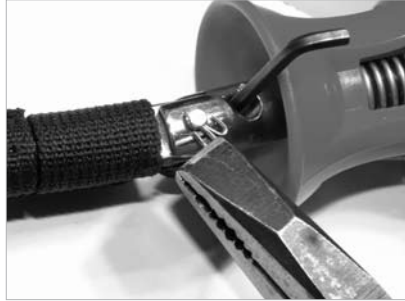
Fig. 14b Use the pliers to pull the cotter pin out.
